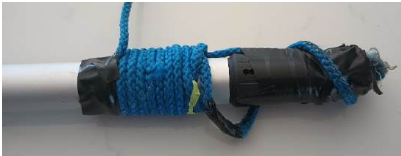
Wrap cord around pole several time and tape
